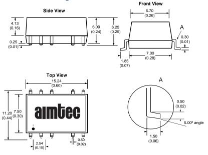
All dimensions are in mm (inch) All Pins are on a 2.54mm (0.10inch) pitch with tolerance of  $\pm 0.25$ mm (0.01inch)
