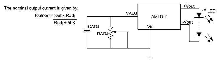
NOTE: Typical error is  $\pm 10\%$  with resistive dimming control If the value of Radj is between 0 to  $2M\Omega$ , the maximum adjustment range will be 25% to 90%, (for Vin –Vout <30VDC)
