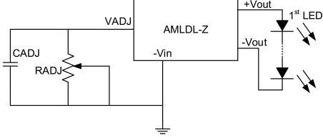
NOTE: Typical error is  $\pm 10\%$  with resistive dimming control If the value of Radj is between 0 to  $2M\Omega$ , the maximum adjustment range will be 25% to 90%, (for Vin –Vout <20VDC)
