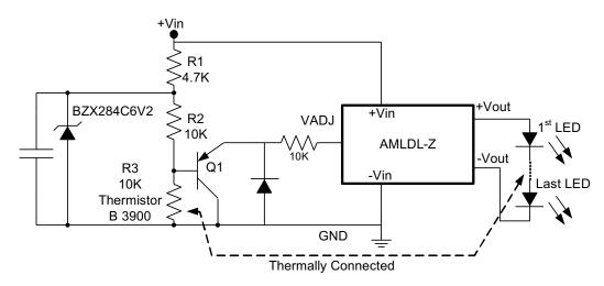
The selection of components for the thermal feedback circuit is depends on the choice of R2 and R3 and the effectiveness of the LED heatsink. To optimize the LED brightness control at high temperatures, the LEDs must have a sufficient thermal extraction path, if not the reduction in drive current will not be optimal.
