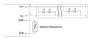
"DO NOT connect "DIM- to -V"
