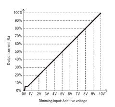
O Applying additive 10V PWM signal (frequency range 100Hz ~ 3KHz):
