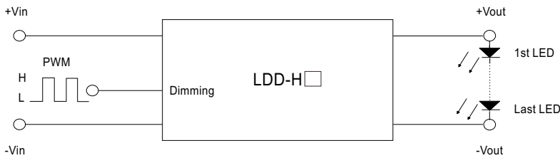
Fig-1 12VDC input, 1~3 LEDs(Vf=3V)
