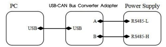
That is: Connect the RS485-L and RS485-H of the signal terminal to the USB interface module When the host computer communication is turned on, you can see the following monitoring screen
