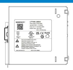
Note: Keep the following installation clearances: 20mm on top, 20mm on the bottom, 5mm on the left and right sides are recommended when the device is loaded permanently with more than 50% of the rated power. Increase this clearance to 15mm in case the adjacent device is a heat source (e.g. another power supply).
