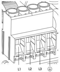
Line size: 24-10AWG Torque: 0.5Nm
