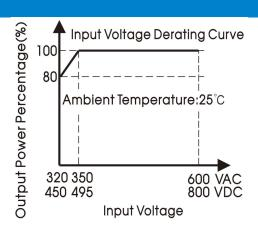
Note: 1. With an AC input voltage between 320 - 350VAC/450 - 495VDC the output power must be derated as per the temperature derating curves;
