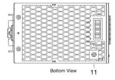
10, 11 any position must be connected to the earth( $\bigoplus$ )
