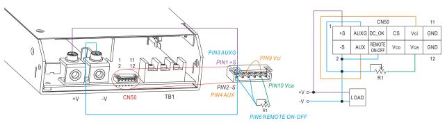
$\bigcirc$  +S & +V and -S & -V also need to be connected on CN50.
