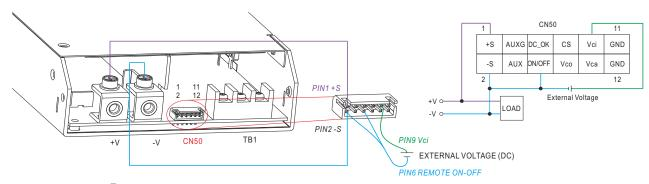
○+S & +V and -S & -V also need to be connected on CN50
