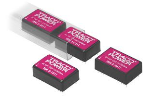
The TEM 2 series is a family of isolated dc/dc converters in a DIP-24 package. They offer tight line/load regulation and 1000 VDC I/O isolation. Standard features include an internal filter to reduce reflected input ripple currrent and to guarantee low output noise. This product series provides a cost effective solution by many industrial or consumer electronics appliactions.
