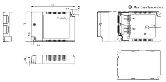
NOTE: Please use wires with a cross section of  $0.75 \sim 1.5$  mm<sup>2</sup> for TB1 and wires with a cross section of  $0.5 \sim 1.5$  mm<sup>2</sup> for TB2.
