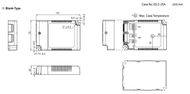
NOTE: Please use wires with a cross section of 0.75~1.5mm<sup>2</sup> for TB1 and wires with a cross section of 0.5~1.5mm<sup>2</sup> for TB2.
